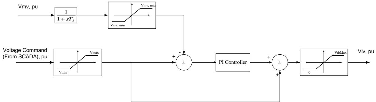
Figure 8: BESS Voltage Control Block Diagram for Islanding Operation Mode
