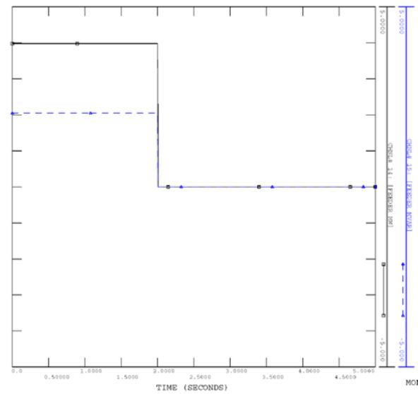
Figure 12: Grid Power Responses in Islanding System Operations (Solid=MW Power, Dashed=MVAR Power)
