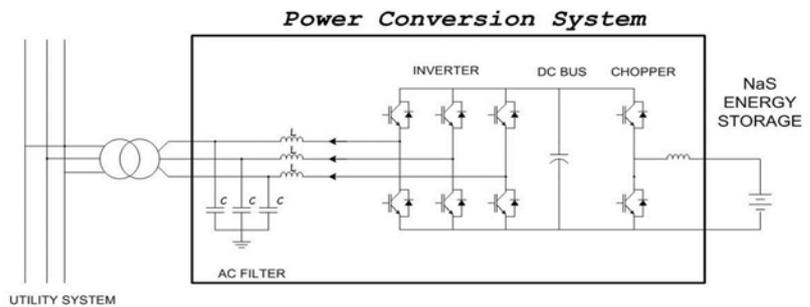
**Figure 2: Single Line Diagram of a Typical BESS**
