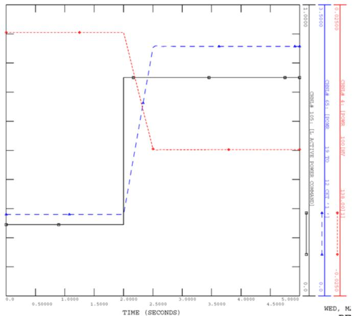
Figure 10: BESS Model Responses (Black=Power Raise Command, Blue=MW Output from BESS, Red=Power Reduction from the Grid)
