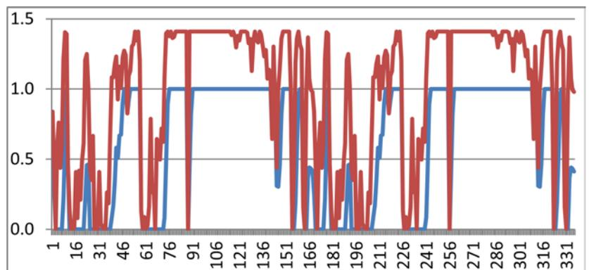
Figure 4: Sample WTG Production Hourly Profile (Red Curve) and BESS Charging and Discharging Operation (Blue Curve)
