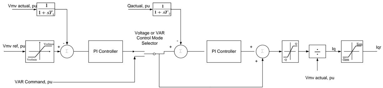
Figure 7: BESS Voltage and Reactive Power Control Block Diagram
