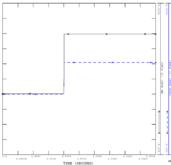
Figure 11: BESS Model Responses in Islanding System Operation (Solid=MW Output, Dashed=MVAR Output)
