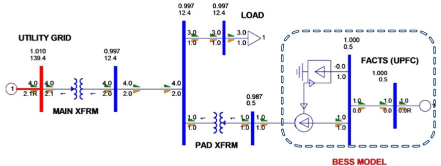
Figure 9: Simplified System with the BESS Modeled as a FACTS (UPFC) Device
