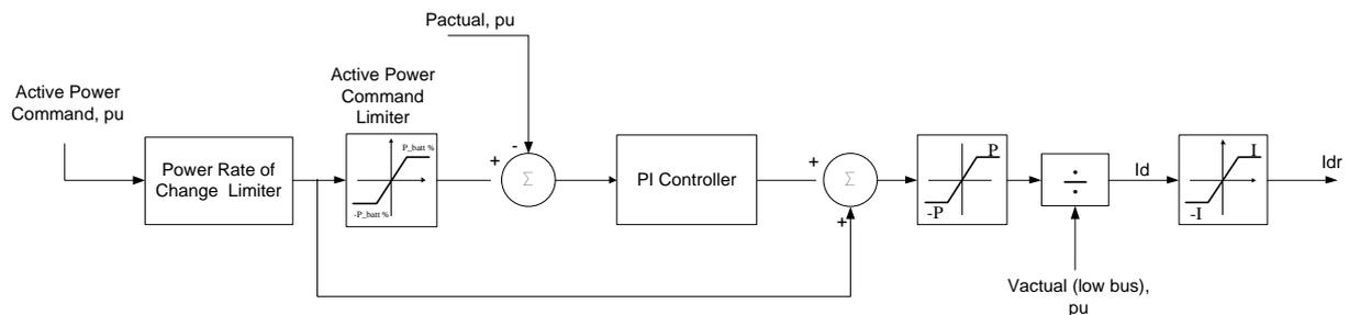
Figure 6: BESS Active Power Control Block Diagram
