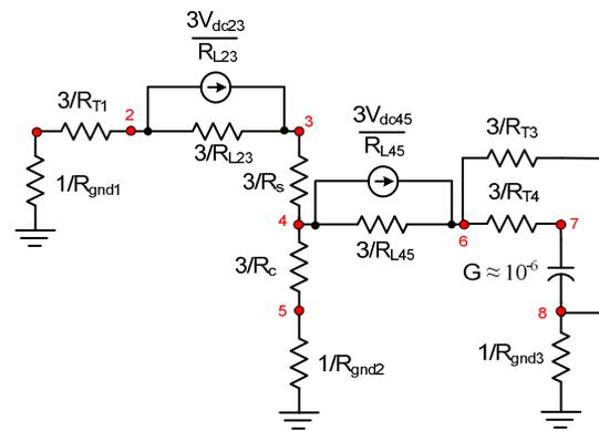
Fig. 6 Norton Equivalent of the dc equivalent circuit provided in Fig. 5.
