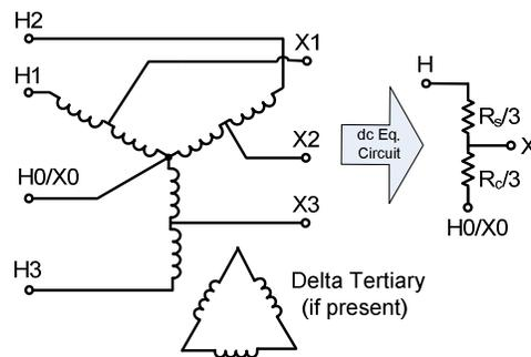
Fig. 3. Single-phase dc equivalent circuit of a two-winding or three-winding autotransformer.
