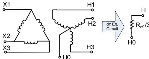
Fig. 1. Single-phase dc equivalent circuit of a GSU.
