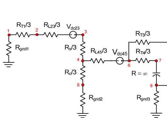
Fig. 5 Single-phase dc equivalent circuit of example system.
