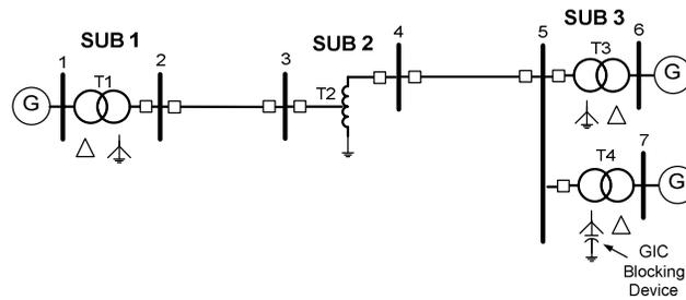
Fig. 4. Example system used to illustrate the procedure of computing GIC in a bulk power system.
