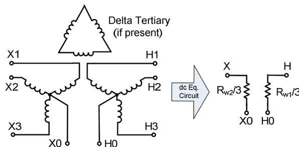
Fig. 2. Single-phase dc equivalent circuit of a two-winding or three-winding transformer.
