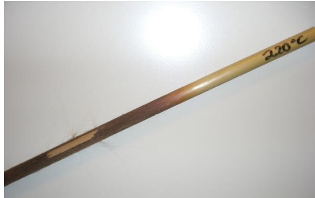
Figure 6 – Composite core sample after 12 month exposure to 220°C
