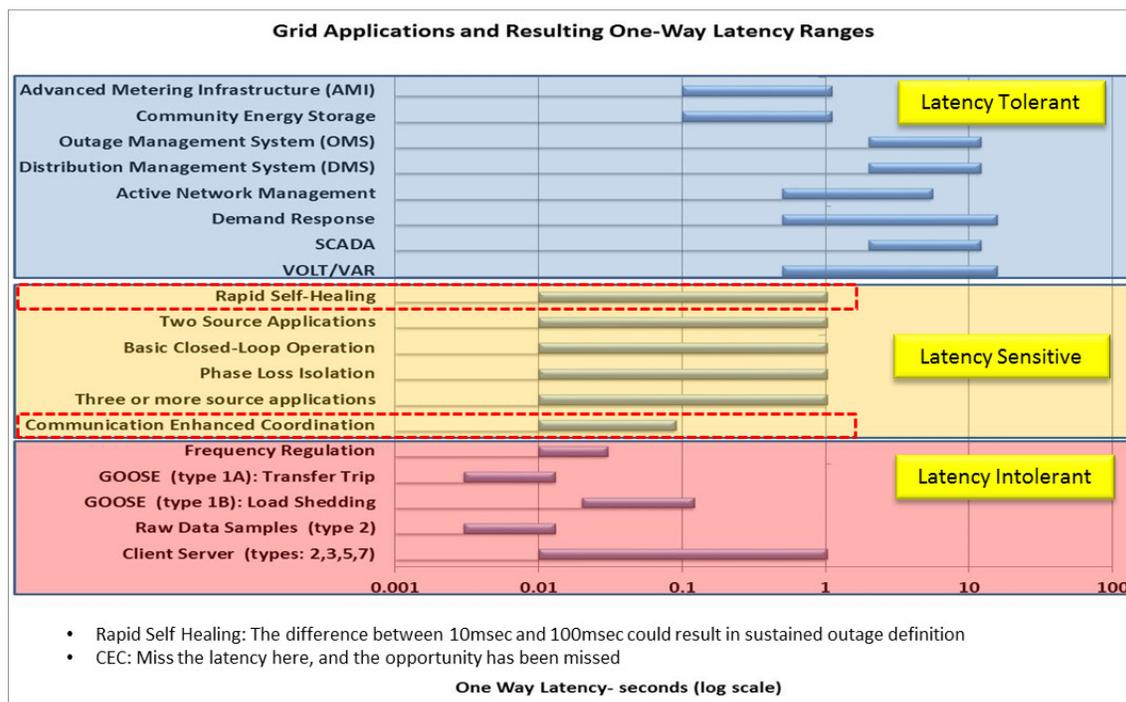
Figure 3. Latency requirements for grid applications
