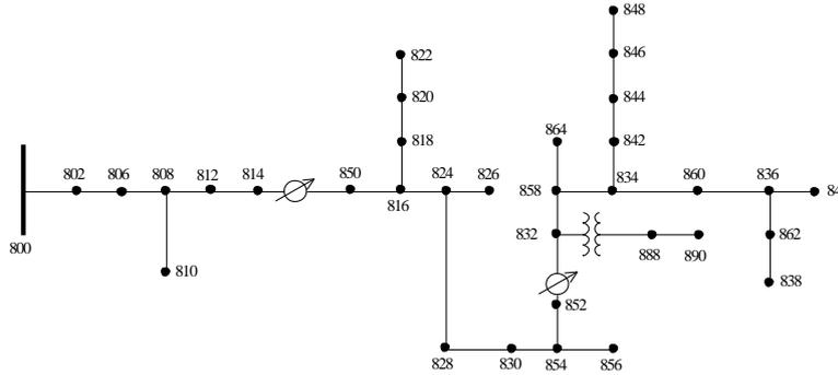
**Fig. 1.** IEEE 34-bus test system
