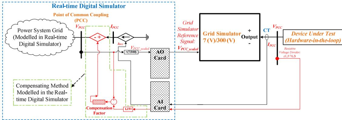
Fig. 7: The proposed PHIL simulation enhanced with voltage feedback
