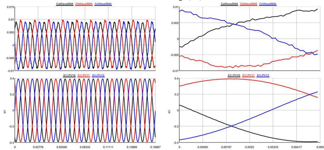
Bus 4; Top: Injected Current (kA), Bottom: Voltage (kV) at the Device under Test (DUT)
