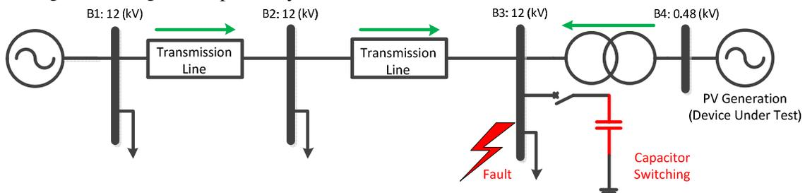
Fig. 9: Single-line diagram of the power system under study and device under test
