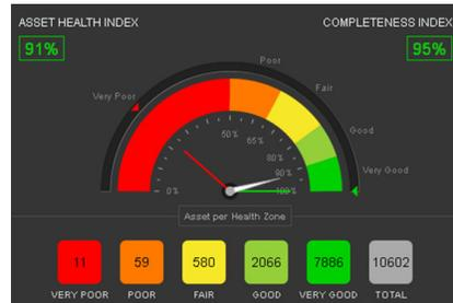
Figure 7: an overall fleet assessment for a part of the grid, showing the split of assets by health zones, immediately highlighting the assets of concern
