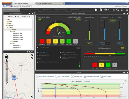
Figure 3: a typical asset health dashboard with the asset navigation tree, geo-referenced displays, analytics presented in synthetic charts for effective decision support.
