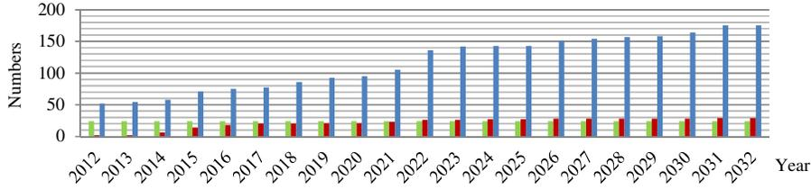
Fig. 1 Planned shunts. Blue: fixed shunt reactor; Red: tap-able shunt reactor; Green: shunt capacitor.
