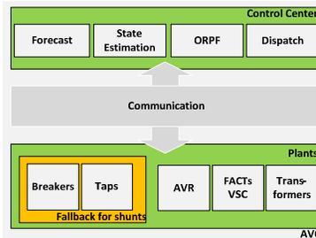
Fig. 3 The Danish AVC system. The control center dispatches the set points to the regulators in the plants via telecommunication networks. The set points are found based on the ORPF algorithm. The fallback controls mainly regulate the shunts locally are activated in case the telecommunications is lost or the voltage violates the defined limits immediate after the AVC dispatches the set points.
