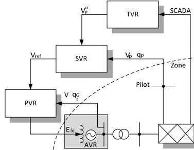
Fig. 2 The general hierarchical structure of AVC system
