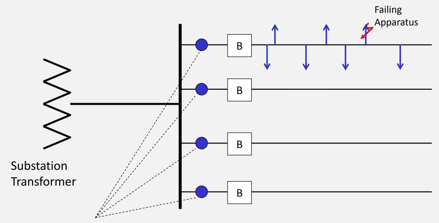
High-fidelity DFA devices, connected to conventional CTs and PTs, one per feeder.
