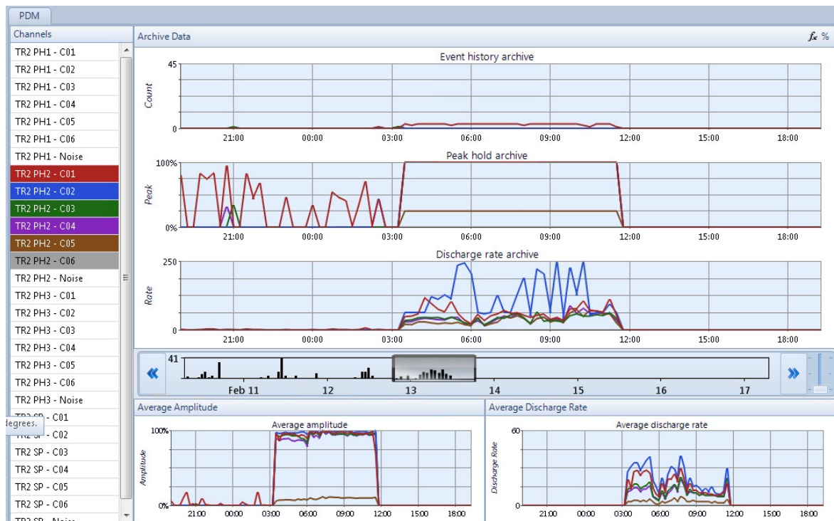
Figure 1: February 2014 Failure Event - UHF Partial Discharge Detection System Data Summary
