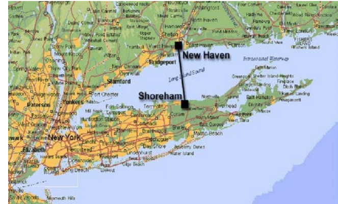
Cross-Sound link between Connecticut and Long Island ( \pm 150\text{kV} , 330MW, 40km)
