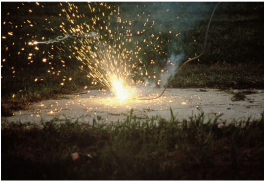
Figure 1: Energized downed conductor ejects molten particles
